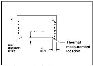
Thermal measurement location – top view
